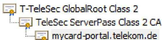
Figure 2: Overview of the certificate hierarchy of the "mycard-portal.telekom.de" web server
